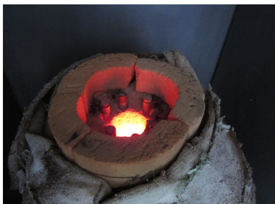
Fig 1. Top view of a reactor using a heat transfer melt for chemical transformations
