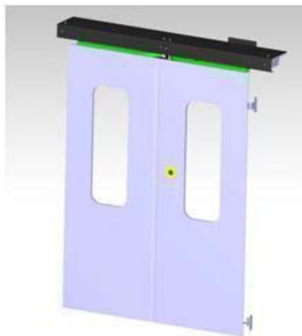
Fig. 1. Designed door system – external view
